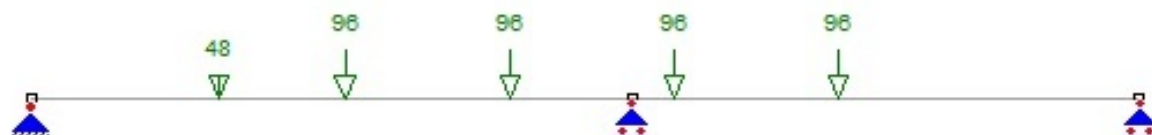
Figure 6- Example of one-dimensional line model analysis of a bridge and heavy vehicle (Each point load represents the total load of an axle)
