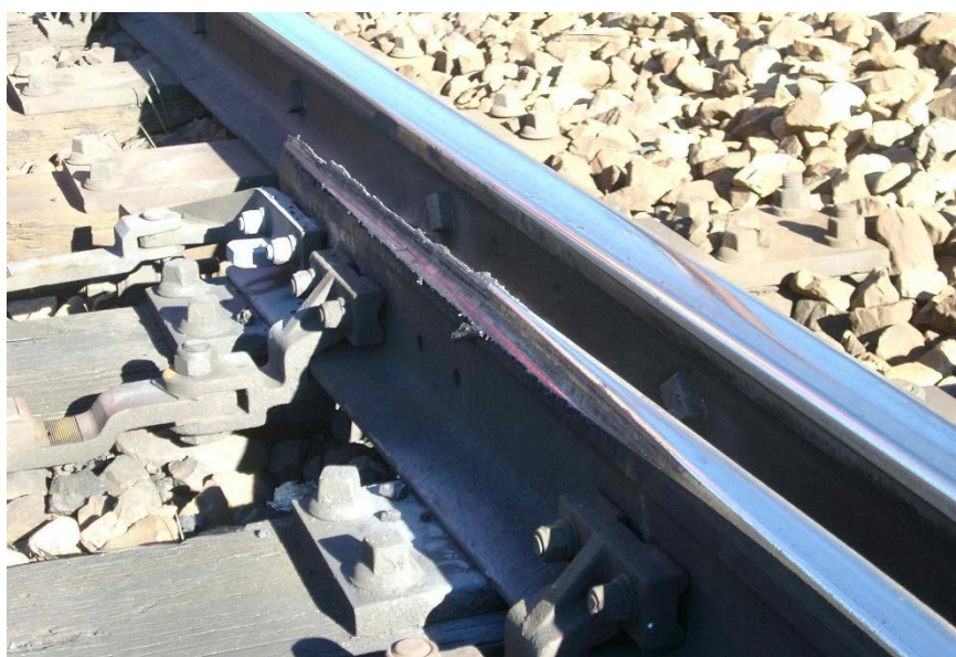
Figure 19 - Example of failure at end of switch
