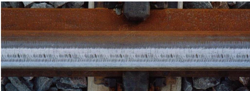
Figure 10 - Example of unacceptable cyclic grinding scratches
