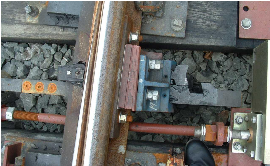
Figure 2.3 – Single Slip, Claw Pinned Directly to Switch Flange
